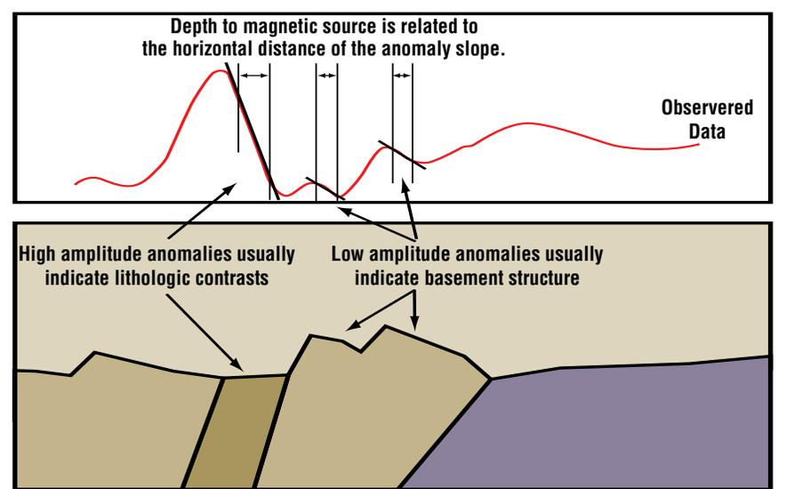
Figure 2: Two-dimensional cross-section
