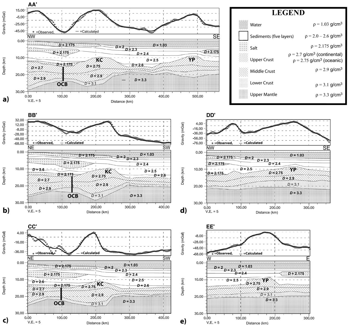
**Figure 5.** Two-dimensional modeled cross sections. All models have the same scale: vertical exaggeration is 5; observed and calculated free air gravity anomalies are dotted and solid lines, respectively. Densities used in modeling are displayed in the legend. The ocean-continent boundary (OCB) is marked with thick vertical lines through upper and lower crust. Models are located in Figures 2 and 3.
